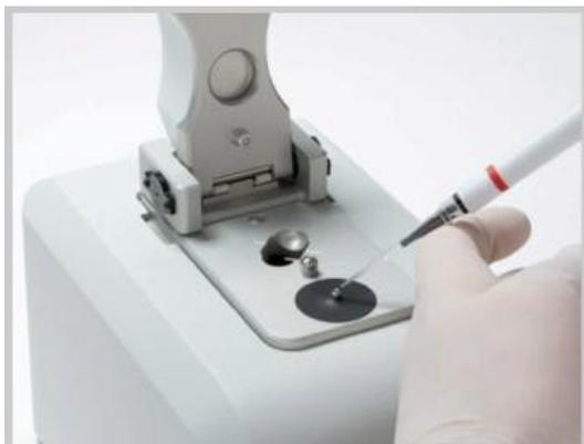
2. Lower the sampling arm and initiate a spectral measurement using the software on the PC. The sample column is automatically drawn between the upper and lower pedestals and the measurement is made.
